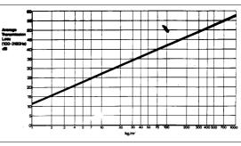
Figs 16 and 17 Sound Transmission of a single partition
